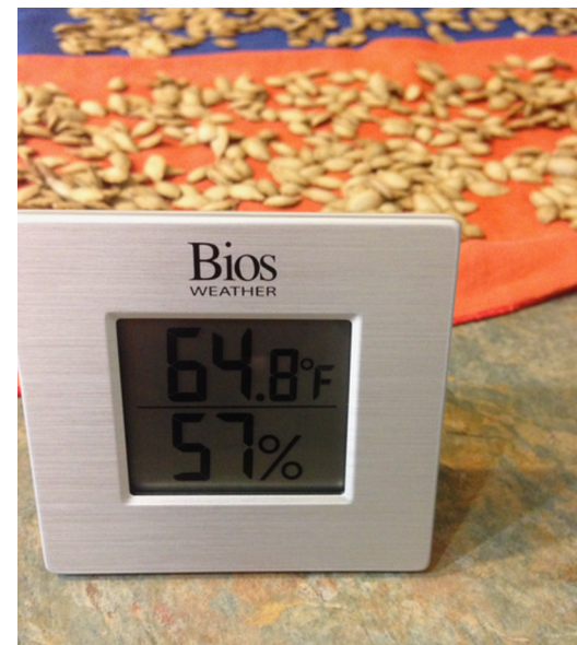
Figure 9: A hygrometer monitors ambient conditions next to drying pumpkin seeds. These numbers exceed the 100 rule and the relative humidity is too high. Seeds need more time to dry, and better drying conditions.
