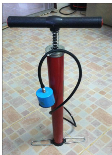
Figure 6. Bicycle tire pump modified for vacuum sealing. Source: ECHO Asia staff.
